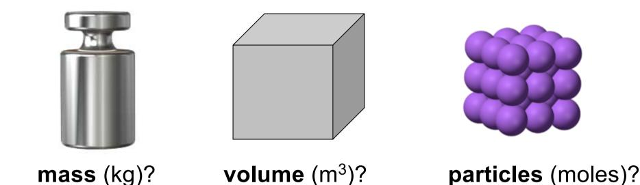
All of these are used to compare heat capacities, but for GCSE we use SPECIFIC Heat Capacity which compares the same amount of MASS. SPECIFIC HEAT CAPACITY (c) is.... How many JOULES of heat energy are needed to raise the temperature of: each kg by each ° C
